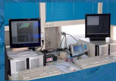
Multibeam Bathymetric System SEABEAM 1050 ELAC – Nautik (180 KHz) DGPS OMNISTAR HP GPS Trimble R3 CEEDUCER PRO – Digital Hydrographic Survey System
